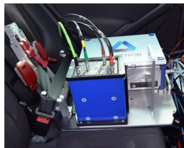
On-seat-adapter for ADMA and data acquisition systems
