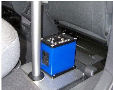
Mounting plate with quick installation mounting pole
