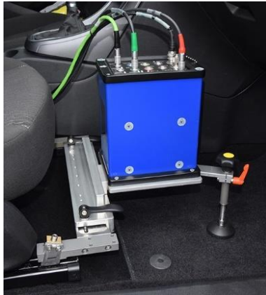
Seat rail adapter with ADMA mounting plate
