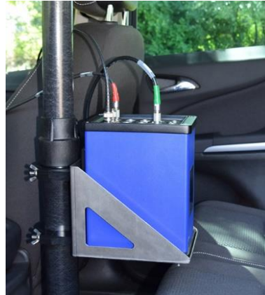
RT-Strut with ADMA mounting adapter
