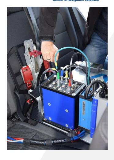
At the heart of the system is the GeneSys ADMA-G-Pro+ GNSS-aided inertial measurement system with its high-performance fiber optic gyros (FOG). It is provided on a quick mount (on-seat adapter for rear seat or passenger seat). ADMA determines the actual trajectory with an accuracy of up to +/- 1 cm, as well as other vehicle dynamic variables such as acceleration, yaw rates, angle and velocity.
