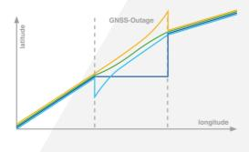
INS Position Forward INS Position Backward INS Position Combined GNSS Position
