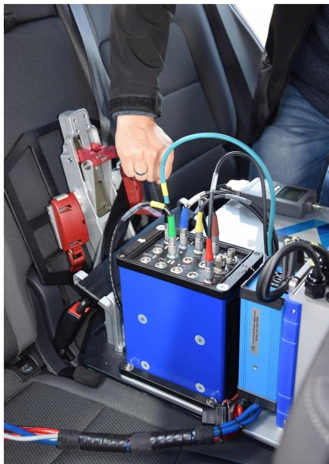
There is also room for the data acquisition (DAQ) on the bracket. Any DAQ system that can record data fully synchronously can be used. Prefabricated plug-ins for the ADMA inertial system, such as those offered by Vector (CANape), digitalwerk (ADTF), DEWESoft and DEWETRON, are practical.
