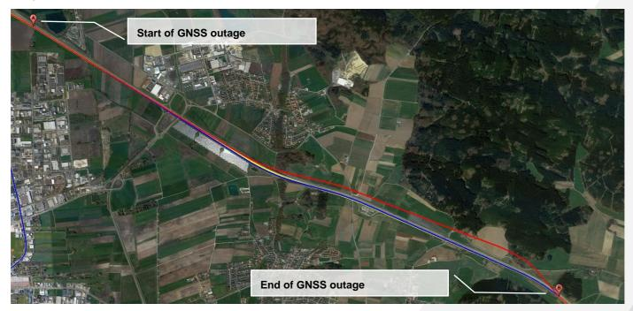
Blue line:Reference drive with ADMA-G-Pro+ without GNSS outageRed line:Signal sequence of live drive during five-minute GNSS outageYellow line:Result from ADMA-PP during five-minute GNSS outage
