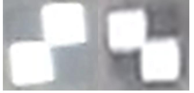
Fig. 2. Shown is a GCP as seen on aerial imagery. The UAV hovers at 50 m (left) and at 100 m (right). The blurring effect of the image prevents to unambiguously assign a pixel to a corner of the GCP.
