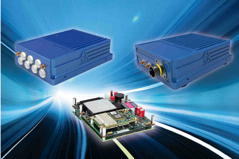
ADMA-Slim is available in three versions: a multi-connector and a single-connector version (both in a waterproof housing) as well as an OEM version.
