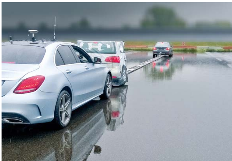
Centimetre-accurate measurement of distances or relative angles between several vehicles e.g. AEB testing.
