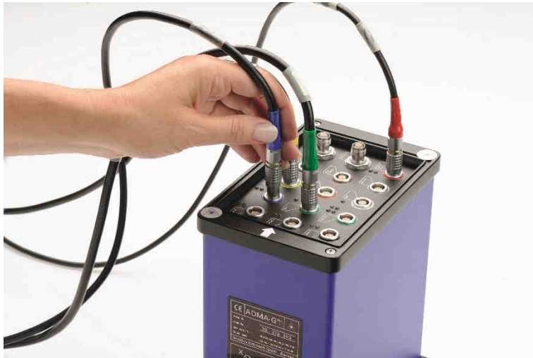
New generation GPS/gyro platform ADMA with an output rate of 1000 Hz
